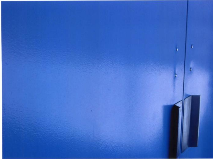
5. Steel faced doors protected with clear GSS-10, Gloss. Note retention of gloss and color after 6 years of exposure.
